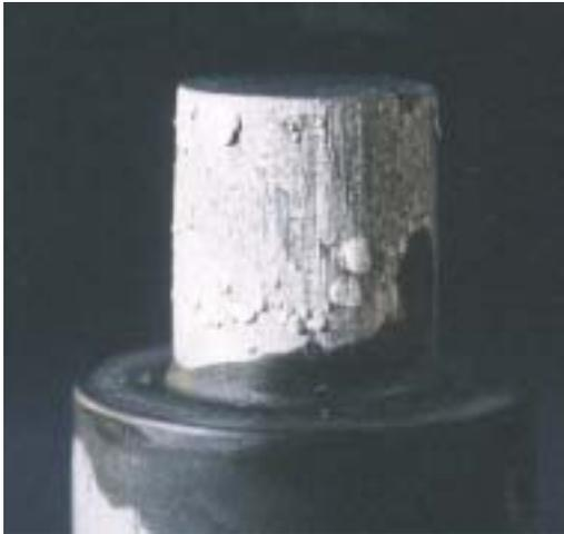
Soldering damage on a core pin.
