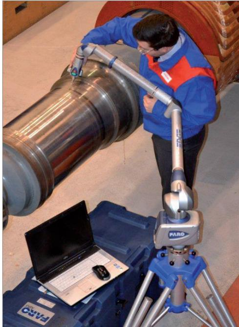
Measurement for checking and redesign of generators or their components to receive a greater accuracy
