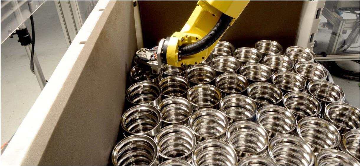
*An automated FANUC robot boxes and palletises parts*
