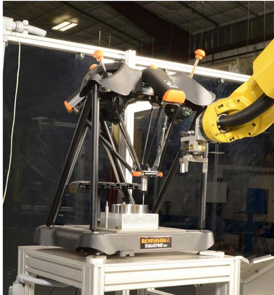
*A FANUC robot loads the Equator in the automated cell*
