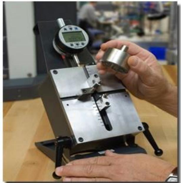
Fig. 2 and 3: Dial Indicators are basically mechanical amplifiers. Digital indicator 1087 R (right)
