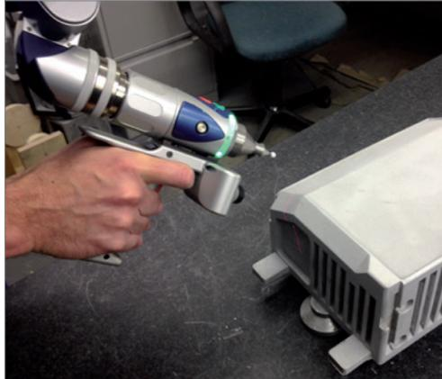
Non-contact measurement of castings to speed up precise inspection routine
