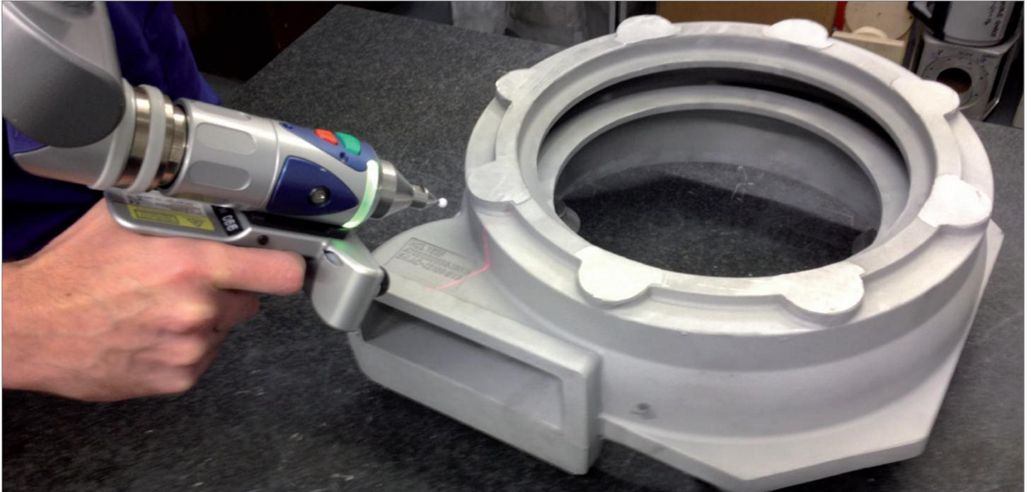
Measurement of precision aluminium castings
