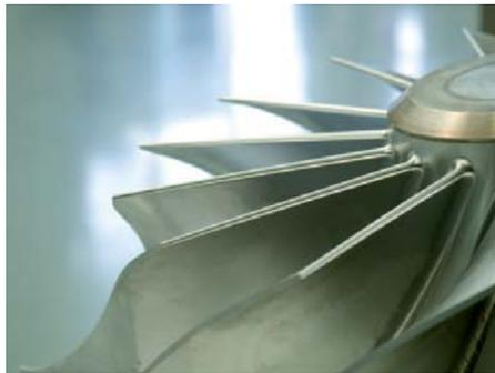
Five-axis machining has long become the standard for the machining of jet engines. High efficiency requirements are driving continuous improvements in the flow characteristics of all jet engine components. The resulting component geometries are very complex and are therefore manufactured exclusively in 5-axis simultaneous milling movements.
