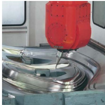
When manufacturing the tool contour, the machine has to maintain a very small distance between cutting paths in order to fulfill the requirements for high surface quality. This automatically lengthens the run times of the NC programs. The required accuracy of the forming tools is a formidable challenge for machine tools: high accuracy during long program run times on large components necessitates high thermal stability of the machine structure and the feed drives.
