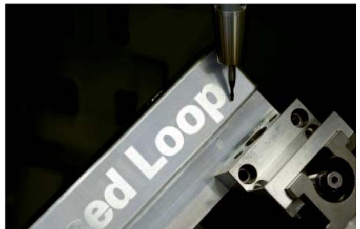
**Closed Loop:** Accuracy-limiting influences from the drive mechanics have no influence on the results of machining. Thanks to the precise angle encoders from HEIDENHAIN, a high contour accuracy and excellent surface definition of the workpiece are achieved.
