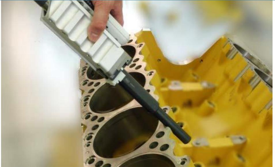
Fig. 3: MarSurf SD 26 with bore fixture
