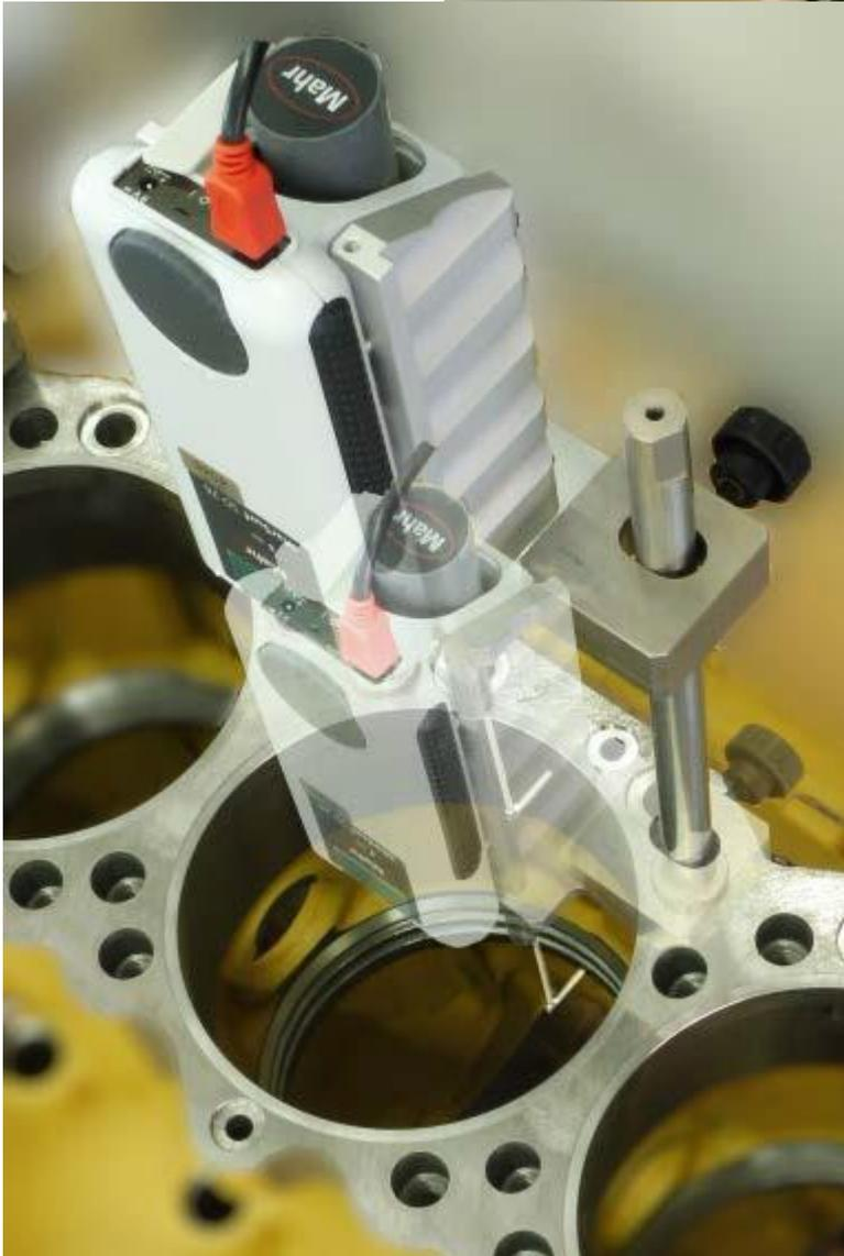
Fig. 4: Roughness measurement in different depths of the cylinder bore with MarSurf SD 26
