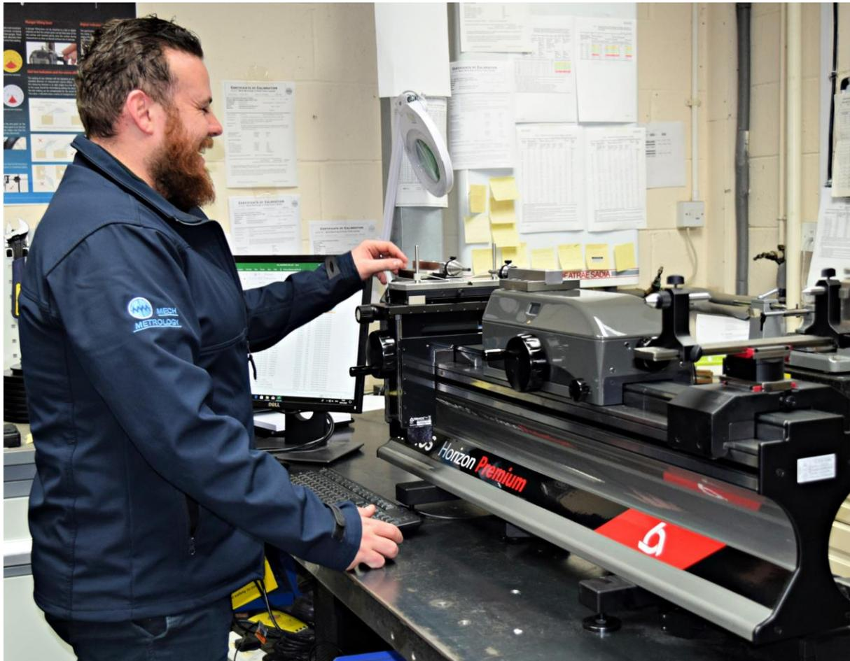
Mech Metrology is now able to test screw ring gauges and internal threads in house, a job that would have been previously subcontracted out. The Trimos Horizon Premium has also improved MECH Metrology's output, as well as significantly increasing the efficiency of the calibration process.
