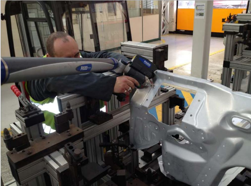
Confirming hole diameter & position to CAD.
