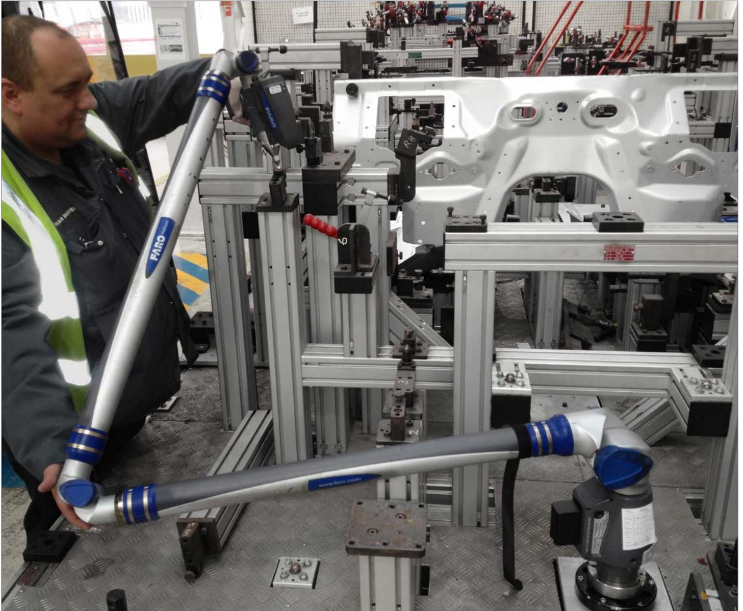
Check of BIW (body in white) panel on PCF (part checking fixture).
