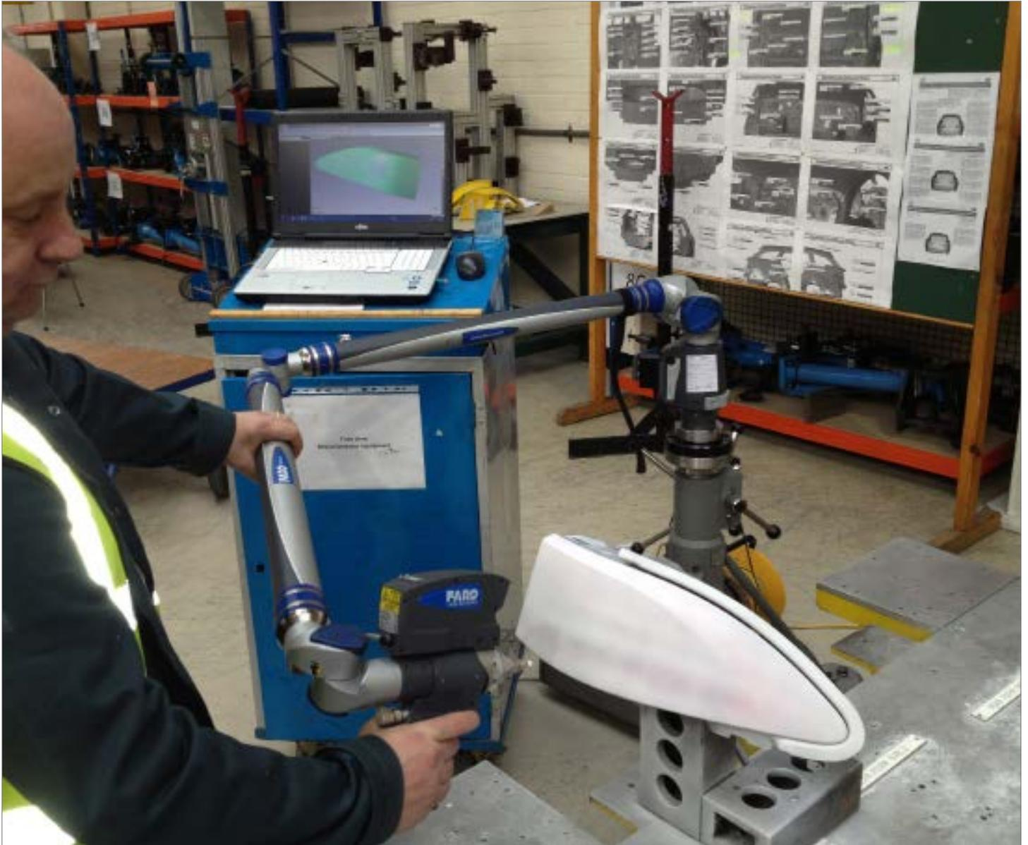
Laser scanning rear lamp cluster for comparison to CAD model.
