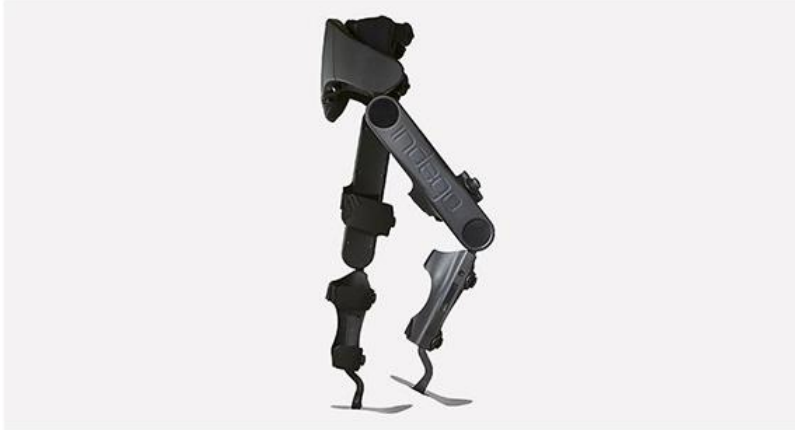
The Indego is a robotic exoskeleton designed to help patients with lower limb paralysis walk again. During development, Parker Hannifin used Protolabs to quickly test design improvements.
