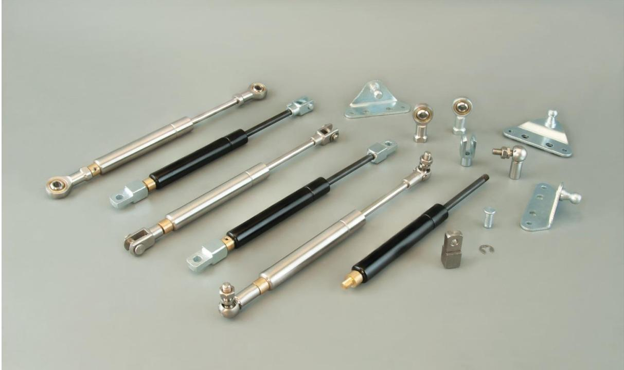
On the WDS website, engineers can specify the required size, stroke length, thread and force of the spring, along with the material of construction. Rod and cylinder sizes range from 6x15mm to 14x28mm, in lengths from 10-1000mm and strokes from 20-500mm. Forces range from 20N to 500N. The products are available in carbon steel or 316 stainless steel.
