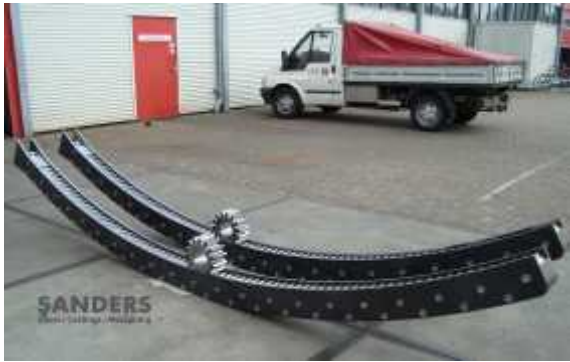
Fig 3 Close up of Curved gear rack for the Redbridge draw bridge manufactured by SANDERS, the Netherlands
