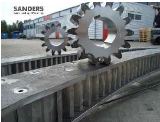
Fig 3 Close up of Curved gear rack for the Redbridge draw bridge manufactured by SANDERS, the Netherlands
