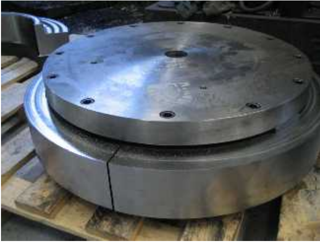
Setup for machining gear ring parts
