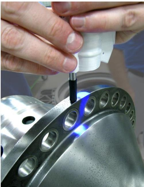
**The 4D INSPEC<sup>®</sup> instant 3D micro-defect inspection gauge** takes the guess work out of 3D micro-measurement, quantifying pits, scratches, nicks, dents, bumps, porosity and other features from 5 $\mu$ m-2.5mm deep over a field of view of 8x8mm.
