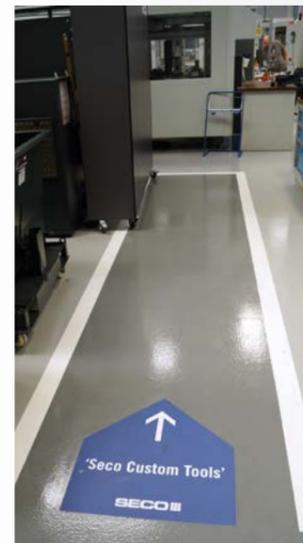
He also explains the rationale behind the installation of the new covers. With the company working to the 5S approach good housekeeping is required as part of a global drive from Seco for its business hubs. Aiming for aesthetic appeal to create a workshop that is closer to laboratory cleanliness rather than an engineering shopfloor environment, where there is a sense of pride in the workplace.
