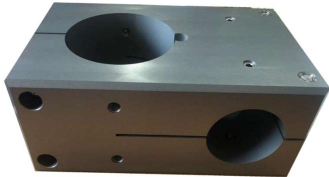
***Main Clamp Block part assembled and Anodized***
