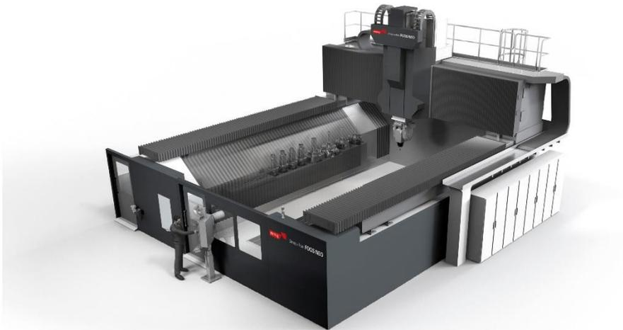
Dynamic and flexible: The Droop+Rein FOGS NEO high-speed machining center with its highly flexible and fast C-axis is ideal for multi-functional complete processing of very large workpieces
