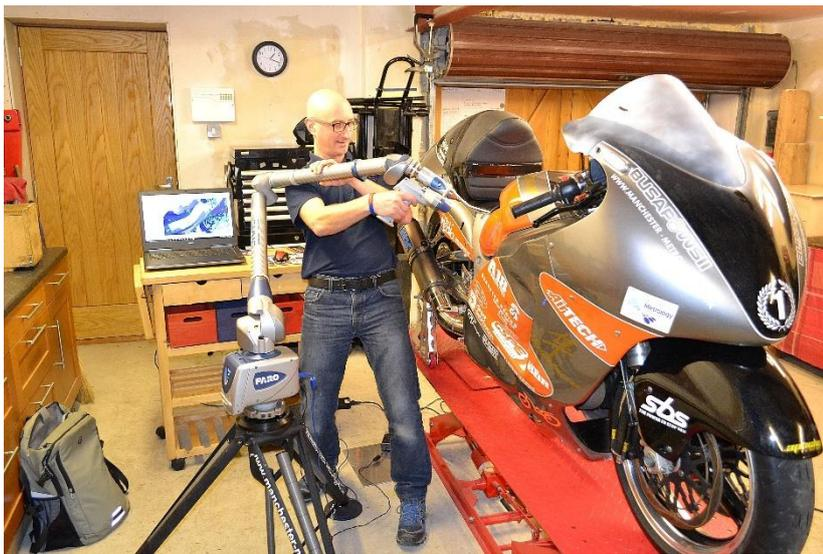
To help gather the raw data needed to enable the best possible virtual simulation outcomes, the team enlisted the help of Manchester Metrology, acknowledged experts in the field of precise laser scanning and data capture. Mindful of the need to acquire highly accurate data, the staff of Manchester Metrology used a FARO Edge ScanArm HD to undertake the critical scanning routines of the bike and rider.
