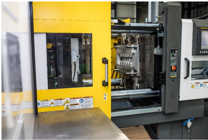
Photo caption: FANUC Electric moulding machine used to produce Kaelo parts
