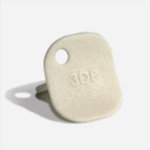
In 3DP an inkjet print head moves across a bed of powder, selectively depositing a liquid binding material, and the process is repeated until the complete part has been formed. After completion, the unbound powder is removed leaving the finished object.
